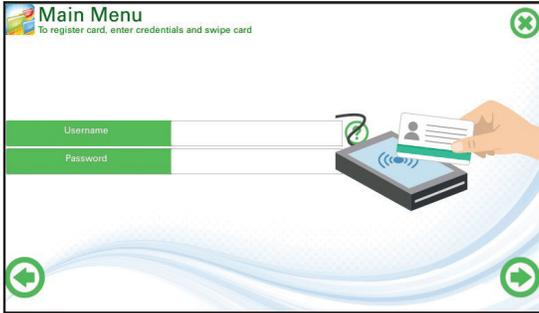
Using the Single Sign-ons authentication feature provides additional security when logging on to the MFP. Users can access the MFP easily with a single card swipe.
